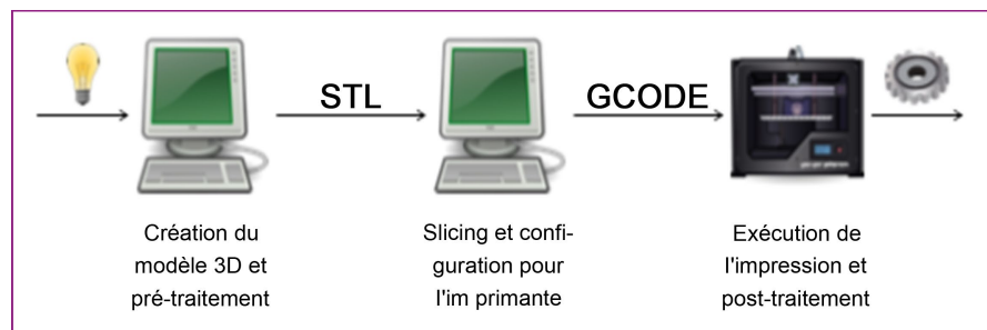
Figure 1. Three-dimensional printing process [6].
