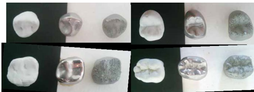
Figure 8. Photographs of plaster reference crowns (left) and polished (middle) and unpolished (right) metal crowns [24].
